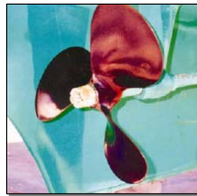
After wiping the propeller off with a wet cloth, the coating shows no deterioration
